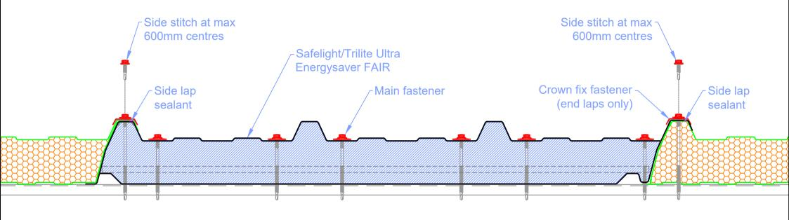
Main fastener - Ø5.5/6.0mm SS fastener fitted with washer with bonded soft seal (Ø19mm; typically Ø29mm)
