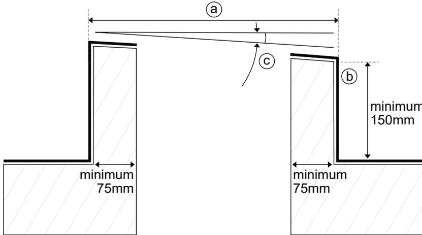
(a) Finished insulated and weathered upstand external dimension: Nominal Rooflight size (+40/-20mm)
