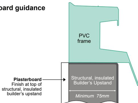
Finish plasterboard at the top of the structural, insulated builder's upstand. Do not cover any of the PVC frame. For more information see TB409.
