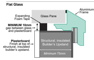
() Finish plasterboard at the top of the structural, insulated builder's upstand, ensuring there is a MINIMUM 10mm gap between the plasterboard and the underside of the glass
