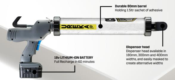
The Cladstikk Gun's innovative dispenser head allows clean and precise application across the width of the cladding boards. Using the correct settings, no adhesive spills over onto the finished substrate and no adhesive is left uncovered. The dispenser heads are available in widths of 180mm, 300mm and 400mm. Dispenser nozzles are disposable and come new with each box of adhesive.
