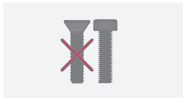
Fig. 12: Avoid screws with countersunk heads
