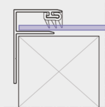
Aluminum F profile available for use where sheet width is reduced, leaving an unsupported edge.
