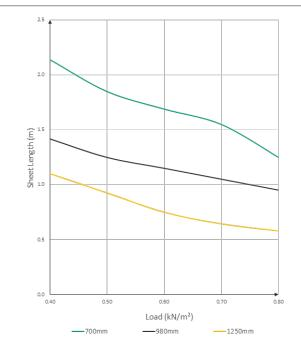
Safe span figures are based on 20mm edge engagement plus a safety factor of 1.2.
